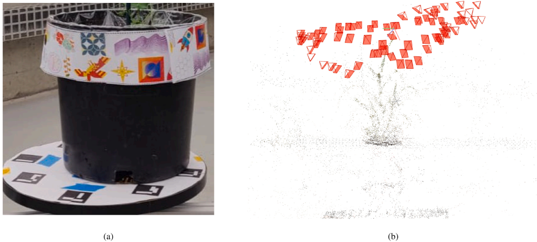
Fig. 3. (a) Plant bucket with colorful tape on corners to improve feature detection; (b) Visualization of GLOMAP-calculated camera poses (red pyramids) representing camera positions and orientations relative to the plant. (For interpretation of the references to colour in this figure legend, the reader is referred to the web version of this article.)
